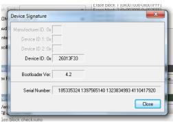
If the communication is working it is possible to proceed with the firmware update. Click on "close" on the "Device Signature" window. In the Flash Magic main window, click on "Start" to begin the programming.
